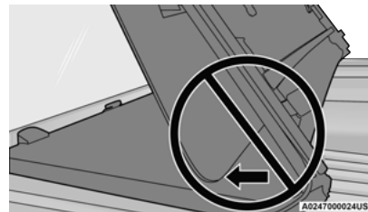
Incorrect Folding — Will Cause Damage
