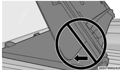
Incorrect Folding — Will Cause Damage
